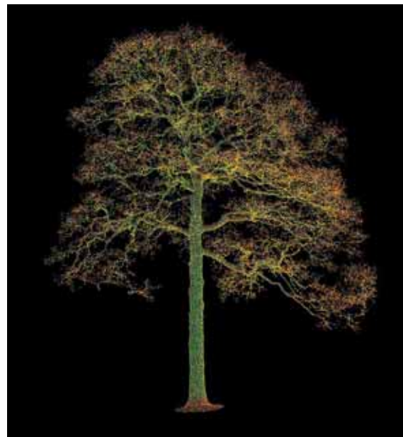
Above: The 3D shape of the tree from the laser scanner 'point cloud'. Scan data processed by Forest Research
